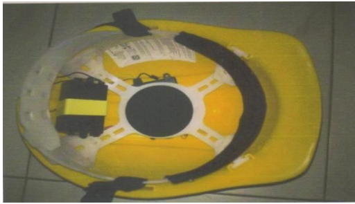
Fig. 7: The Module fitted inside a Safety Helmet
